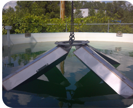
The Fold-a-Float begins to self-deploy as it meets the surface of the water.
